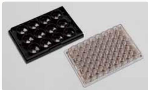
Microelectrode arrays (MEAs) consist of a grid of tightly-spaced extracellular electrodes, each capable of simultaneously monitoring the activity of multiple cells non-invasively. Having multiple electrodes in an array extends the recording range across a relatively large area, revealing detailed information about systems-level signal propagation.
