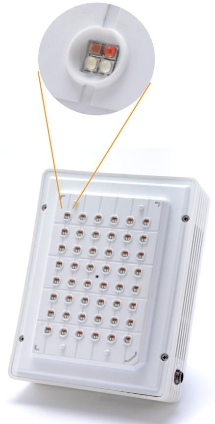
Lumos enables high-throughput optical stimulation in an innovative 48-well format. Each well contains 4 LEDs (inset), used independently or in combination.
